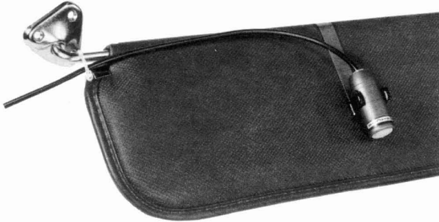
MICROPHONE IN MOUNTING CLIP FIGURE 2
