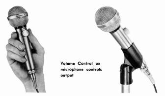
by the main volume control at the amplifier location —then the user can adjust the volume up or down at the microphone position. Maximum volume occurs when the dot on the knob is adjacent to the dot on the microphone (12 o'clock position). In many instances, minimum setting of the volume control will reduce volume sufficiently so that the volume control can be used as an On-Off switch.
