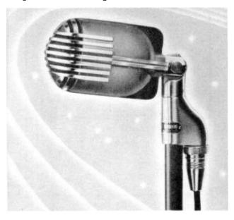
Low impedance models 508A and 508B may be fed into a standard low impedance input amplifier (as into a standard low impedance input amplifier (as shown in Fig. A-3) or into an amplifier with high impedance input (Fig. A-2). In the latter case Shure Model A86A Cable-Type Transformer is available for coupling the low impedance line to amplifier. The double-winding primary permits coupling a 35-50 ohm line or 200-250 ohm line to the high impedance Input of the amplifier.
