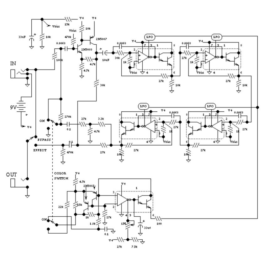
The Small Stone is somewhat unique in using Operational Transconductance Amplifiers (OTA's) for phase shift stages instead of opamps with variable resistors. All of the IC's are house marked EH1048, but can be replaced with CA3094 which is a combination of an OTA equal to the CA3080 and a darlington emitter follower. Later Small Stones used slightly different circuits, but all used the OTA.
